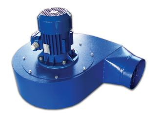
ZWR fans have been designed to work with source capture devices as well as with clean or polluted air extraction installations. Aluminium impellers enclosed in steel powder coated housings ensure high airflow efficiency and sparkproof design. ZWR fan units are used to exhaust non-explosive and chemically non-aggressive gases of temperatures up to 40°C.
